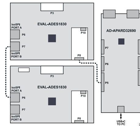
Figure 3. Reverse isoSPI/SPI Connection to the Top
