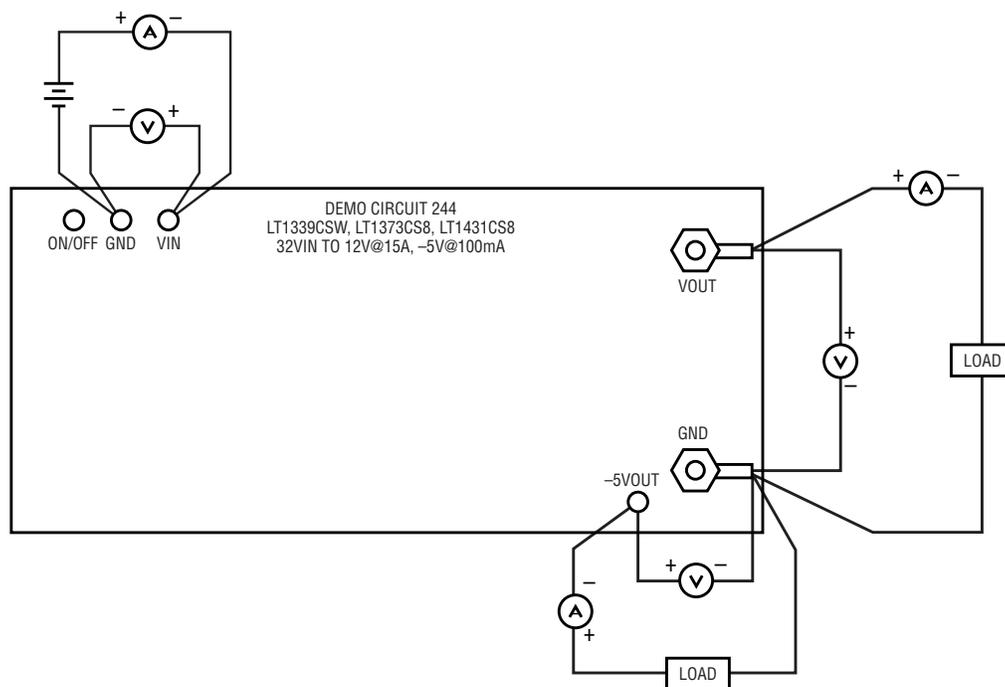
Figure 2. DC244 Proper Measurement Setup
