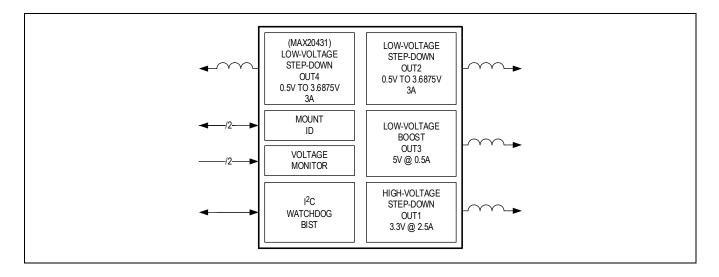
Four-/Three-Output Mini PMICs for Safety Applications
