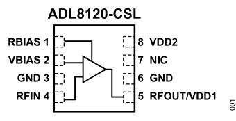
Figure 1. Functional Block Diagram
