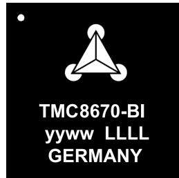
Figure 32: TMC8670-BI device marking
