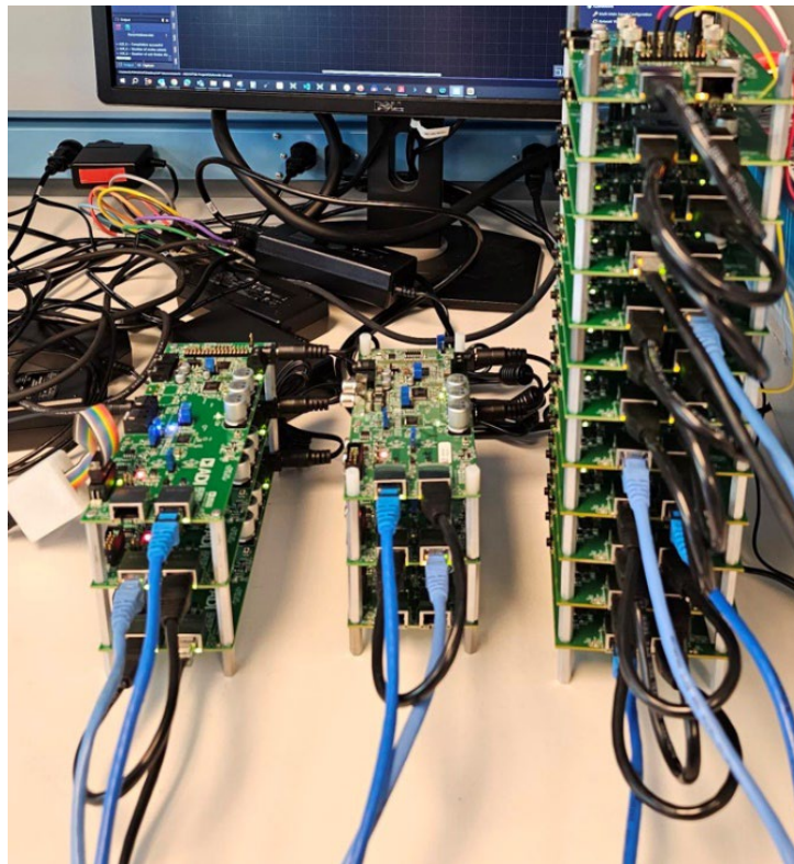
Figure 6 THD+N Test setup using a combination of EVAL-AD2437A1MZ and EVAL-AD2437B1MZ
