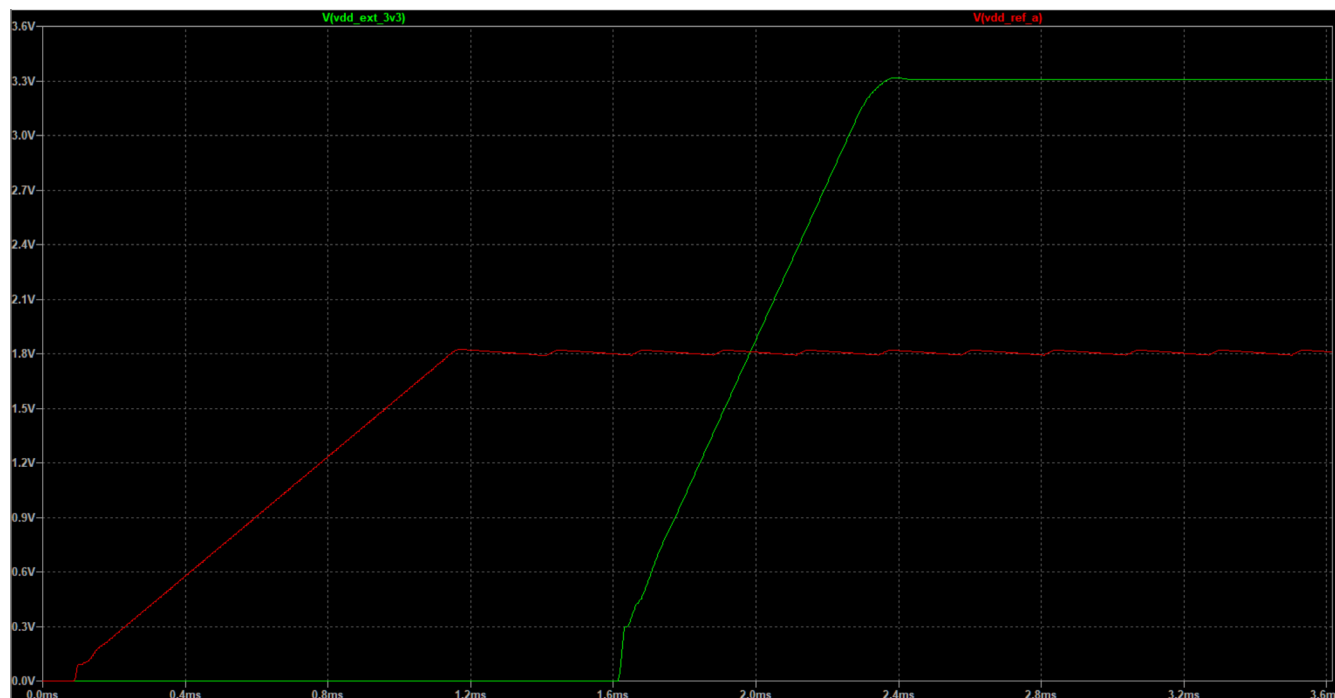
Figure 9: VDD_REF Ramp-up Followed by VDD_EXT
