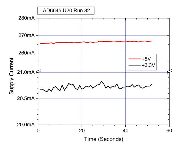
Figure 5.3. Supply current on versus time for AD6645 unit number U20 (Run 82). The testing was performed at an effective LET of 83MeV-cm<sup>2</sup>/mg using Xe at an energy of 10MeV/n. As seen in the figure, the supply current shows no significant increase during the run, indicating that the units-under-test have not experienced a latch-up event.
