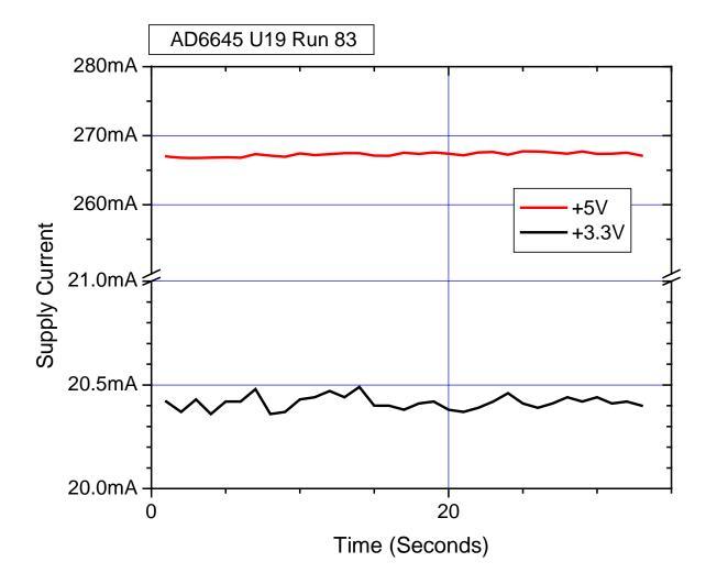
Figure 5.4. Supply current on versus time for AD6645 unit number U19 (Run 83). The testing was performed at an effective LET of 83MeV-cm<sup>2</sup>/mg using Xe at an energy of 10MeV/n. As seen in the figure, the supply current shows no significant increase during the run, indicating that the units-under-test have not experienced a latch-up event.
