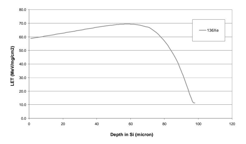
Figure 3.1. Range of the 10MeV/n Xe beam into silicon. The range to the Bragg Peak is approximately  $60\mu m$  while the surface LET is approximately 58MeV-cm2/mg.
