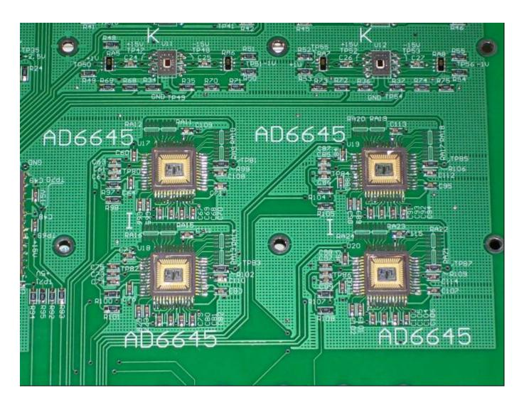
Figure 4.1. Single event test board mounted on the test stage at Berkeley. The board has four units-under-test mounted simultaneously to minimize vacuum breaks during testing. There is also a heater plate mounted to the backside of the board to provide the elevated temperature required for this testing.
