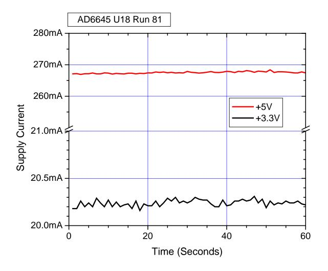
Figure 5.2. Supply current on versus time for AD6645 unit number U18 (Run 81). The testing was performed at an effective LET of 83MeV-cm<sup>2</sup>/mg using Xe at an energy of 10MeV/n. As seen in the figure, the supply current shows no significant increase during the run, indicating that the units-under-test have not experienced a latch-up event.
