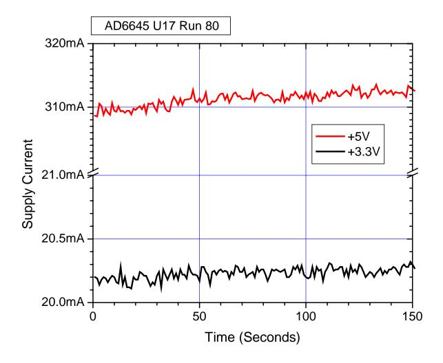
Figure 5.1. Supply current on versus time for AD6645 unit number U17 (Run 80). The testing was performed at an effective LET of 83MeV-cm<sup>2</sup>/mg using Xe at an energy of 10MeV/n. As seen in the figure, the supply current shows no significant increase during the run, indicating that the units-under-test have not experienced a latch-up event.
