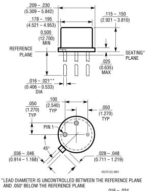
\*\*FOR SOLDER DIP LEAD FINISH, LEAD DIAMETER IS  $\frac{.016 - .024}{(0.406 - 0.610)}$
