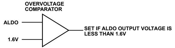
Figure 120. Analog LDO Monitor
